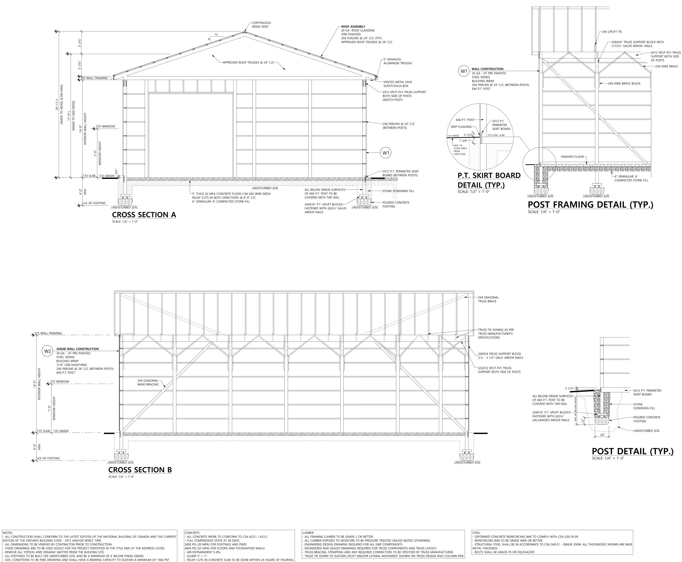
(75 KPA) AND BE VERIFIED BY A LOCAL PROFESSIONAL. - BACKFILL TO BE COMPACTED IN 6" LAYERS. - NO BUILDING SHALL BE BUILT ADJACENT TO OR IN PROXIMITY TO THE STRUCTURE SO AS TO ADVERSELY ALTER WIND OR SNOW LOADING CONDITIONS.
