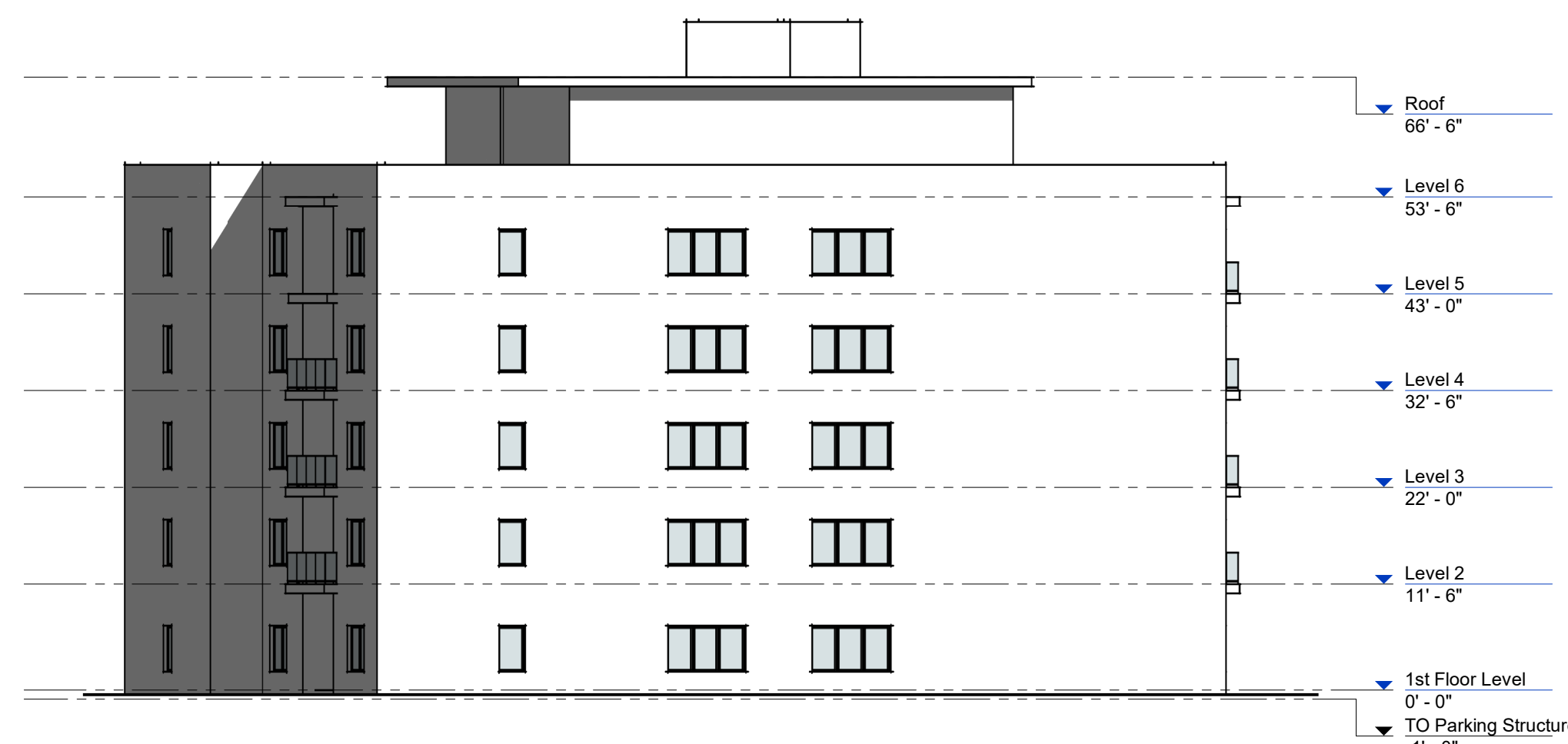
Elevation - West scale: 1/16" = 1'-0"
