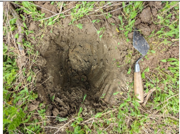
Photo 4: Typical Test Pit
