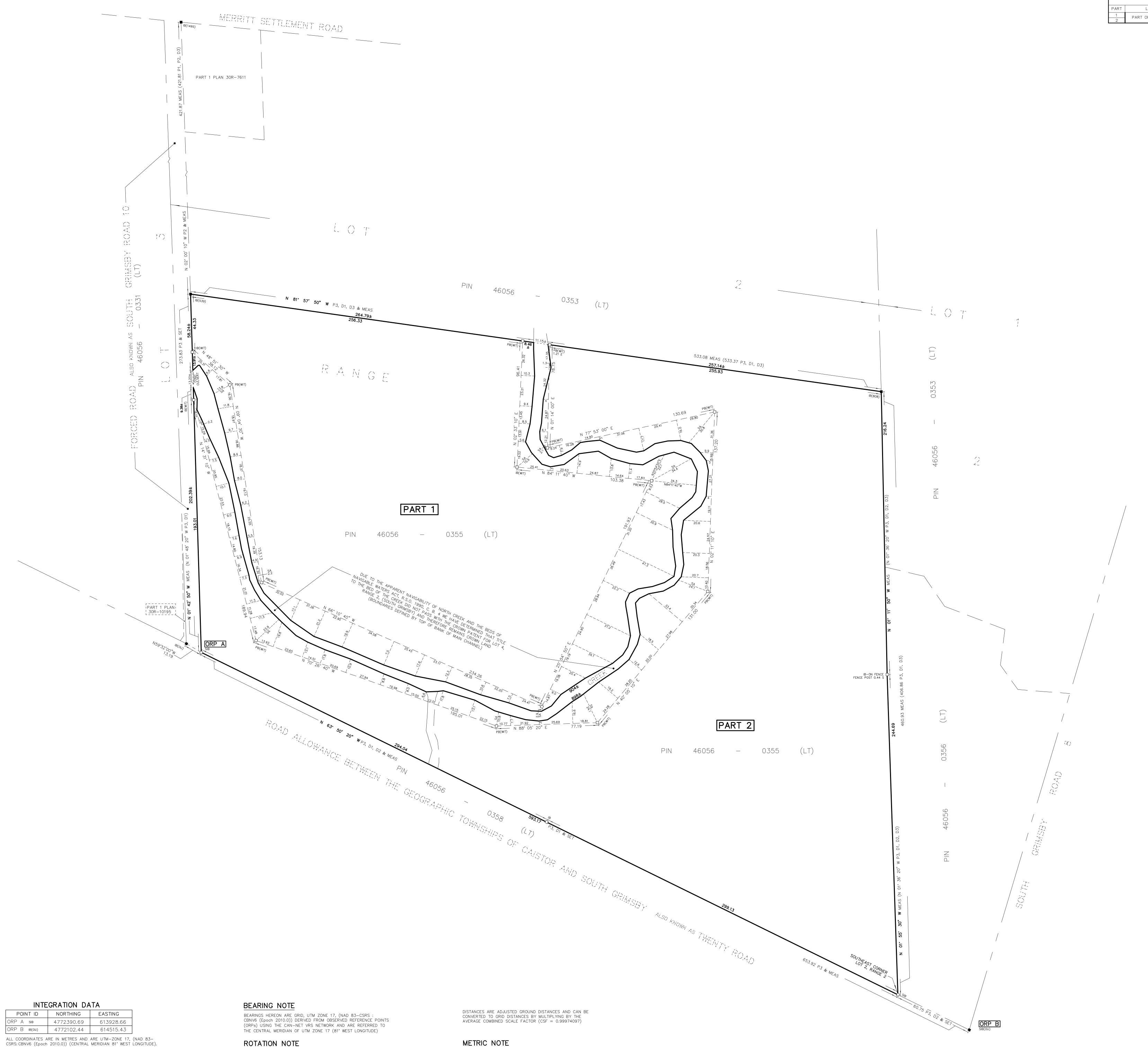
ALL COORDINATES ARE IN METRES AND ARE UTM-ZONE 17, (NAD 83-CSRS:CBNV6 (Epoch 2010.0)) (CENTRAL MERIDIAN 81' WEST LONGITUDE). COORDINATE VALUES ARE TO AN URBAN ACCURACY IN ACCORDANCE WITH SECTION 14 (2) OF O. REG 216/10. CAUTION
